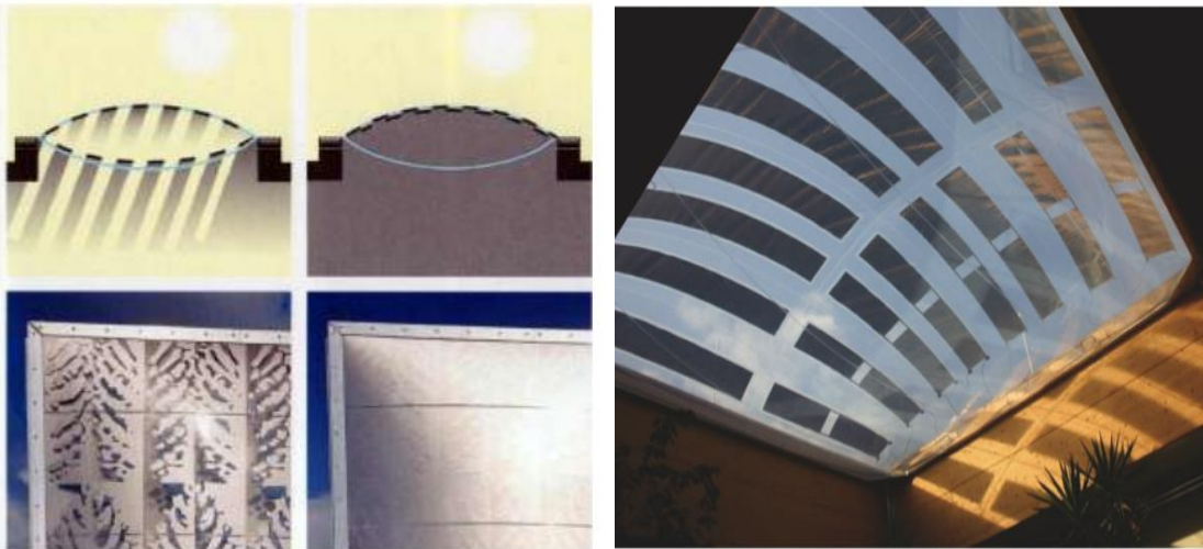
Variable printing patterns and materials (PV) on ETFE membranes
